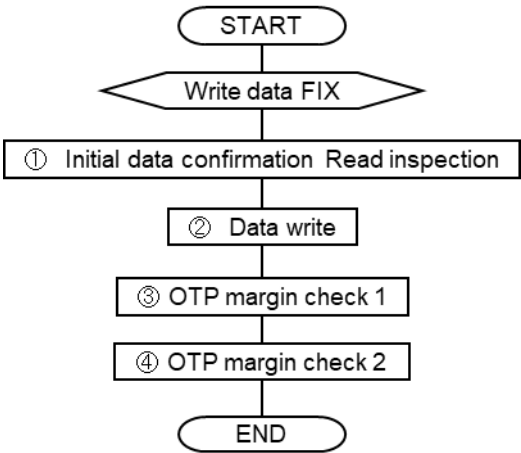
Fig. 4-52 OTP inspection flow
